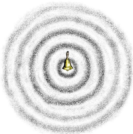
This illustration is not a complete picture because sound waves propagate in three dimensions, not two like the illustration on this paper. This illustration does show that the pressure between the compressions and rarefactions is more pronounced closer to the sound source. The energy carried by the sound wave becomes more spread out the farther the wave is from the source. Some energy is also transformed to heat due to the friction between air molecules.
