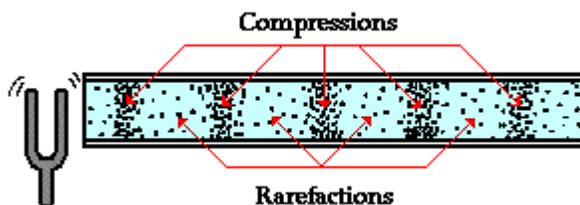
**Compressions** are areas where there is high pressure of air particles and **rarefactions** are areas where there is a lower pressure of air particles.
