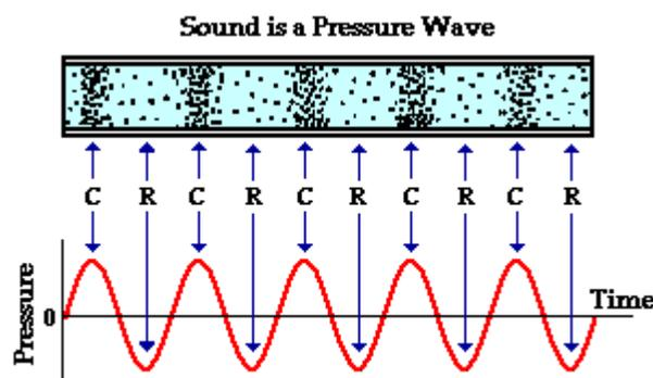
The highest points of the sine wave correspond to compressions; the low points correspond to rarefactions; and the "zero points" correspond to the pressure that the air would have if there were no disturbance moving through it.
